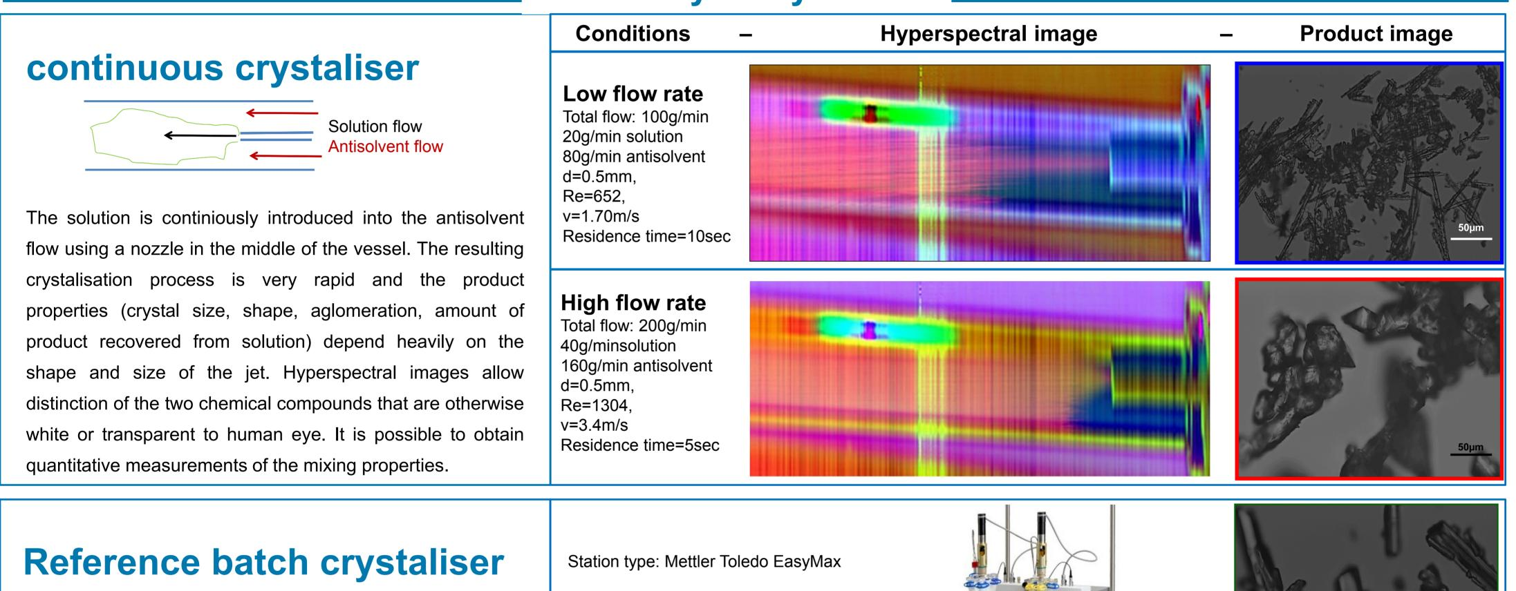
For comparison, the same pharmaceutical was crystalised in a batch crystaliser. The resulting product is shown in the microscopic image to the right. Total volume :100ml Stir rate: 400rpm, Cooling: 1°C/min
