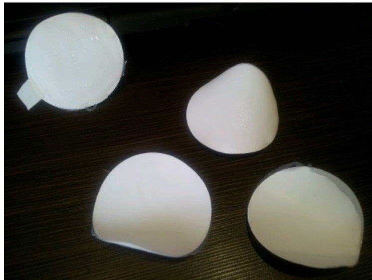
Manufactured air-transducer matching layers
