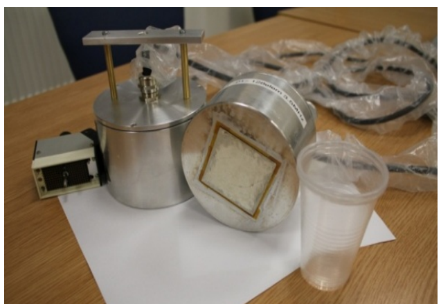
Completed 2D phased array probe, active sensing area diameter 50mm.
