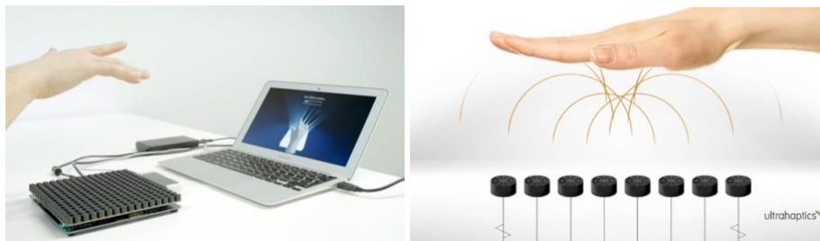
Figure 5: Ultrasonic phased array generating a focus point
